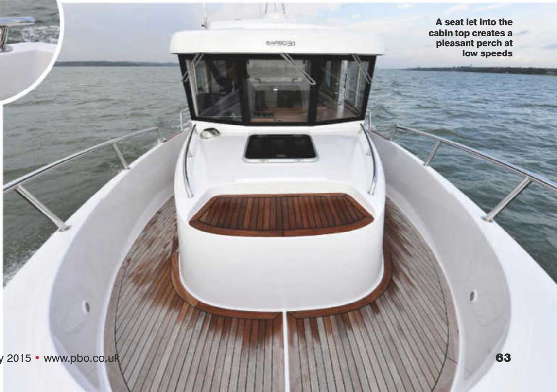
Wide, deeply bulwarked side decks make this a very easy boat to work
