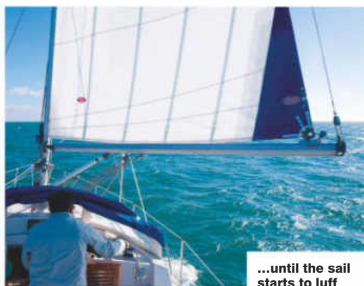
The boat is on a close reach and Owain eases the main sheet...
