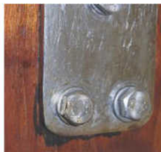
This chainplate and bulkhead have seen some water ingress
