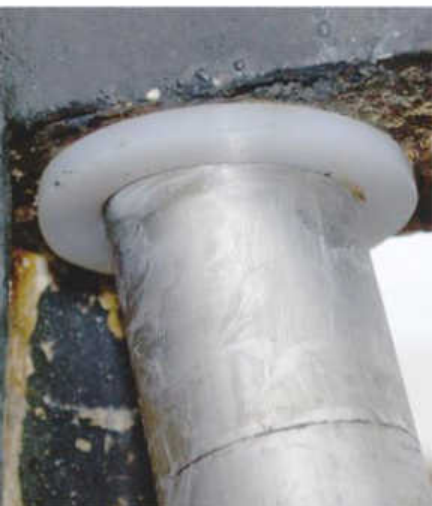
The new bush in place, but with the stock not yet aligned
