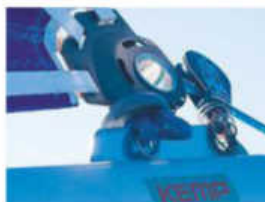
A donut at the clew keeps the sheave from making contact with the outhaul slider
