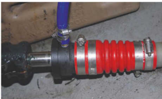
Modern stern glands shouldn't leak, but stuffing boxes are designed to drip
