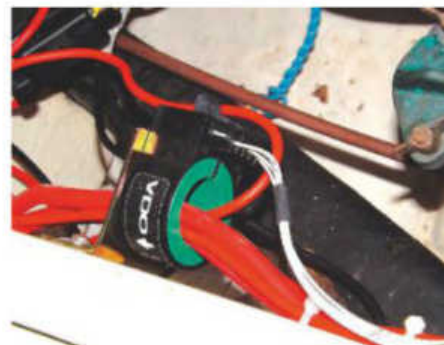
Cables from the alternator and other sources of charging are passed through the Hall effect sensor aperture
