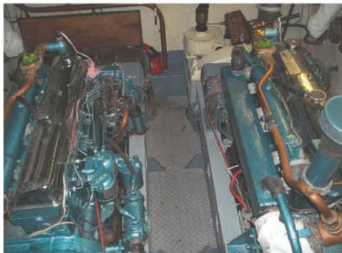
The original engines were replaced with 70bhp Ford Mermaid diesels
