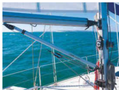
Here's the gas kicker, and the drum for the endless furling line
