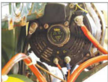
Rev counter connection on the back of the alternator
