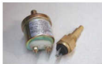
Oil pressure and coolant temperature senders with integral alarm switches
