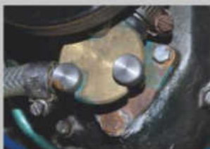
This water pump has been leaking, as shown by the rust
