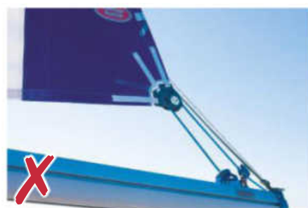
The clew should be close to the boom, not way above it like this
