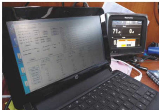
RS11 over-temperature alarm set via the utility software. This is set to around 85°C as an early warning
