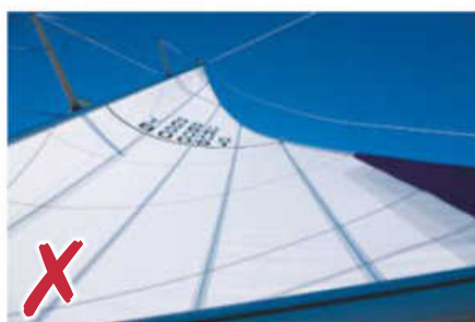
Too much twist (not enough kicker tension) and too little outhaul results in an inefficient shape
