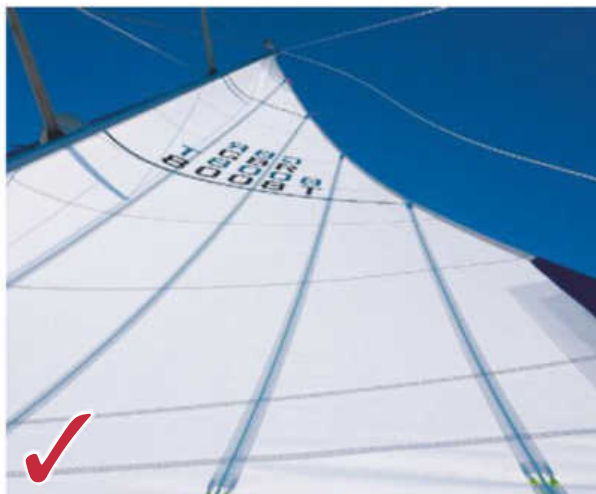
Here's a nicely set sail for fresh conditions, with the right amount of twist (top telltales flying)...
