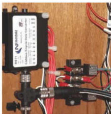
RS11 fully installed and connected to the Raymarine backbone via the DeviceNet to STNG cable adapter
