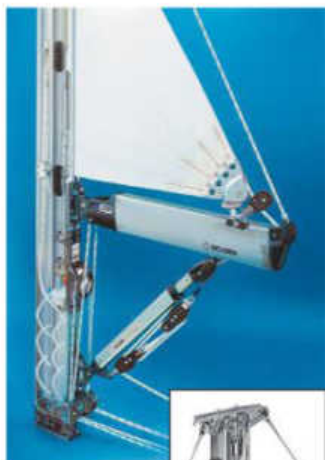
For the past 15 years or so, Seldén's Furlin RB system has used a tensioned luff spar with a bearing at the top and a bottlescrew at the bottom
