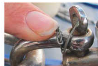
Seize shackle pins to prevent them from working loose
