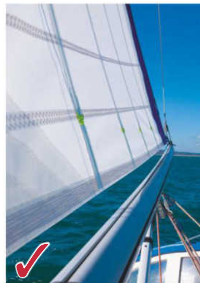
...and a tight foot, which you need in any breeze. Ease it on a reach or in less wind
