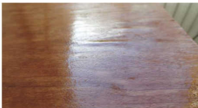
This veneer buckled badly 24 hours after a second coat of varnish
