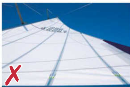
Here the kicker is too tight and there's not enough twist (top telltales stalled)
