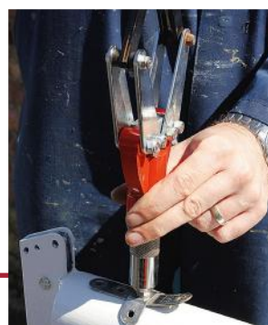
The spinnaker pole uphaul fitting is riveted onto the mast
