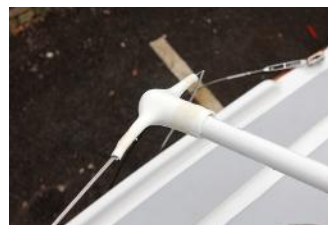
These Plastimo spreader boots will stop chafe and sail damage shroud, which is secured with good old-fashioned seizing wire.
