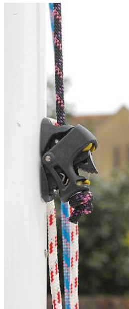
ABOVE Our new pole downhaul arrangement, which uses a Barton size 2 block with cam cleat
