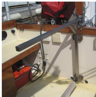
SALOON/COCKPIT TABLE Uses the same brackets and support for the table in the cockpit as in the saloon. Table stows beneath the foredeck
