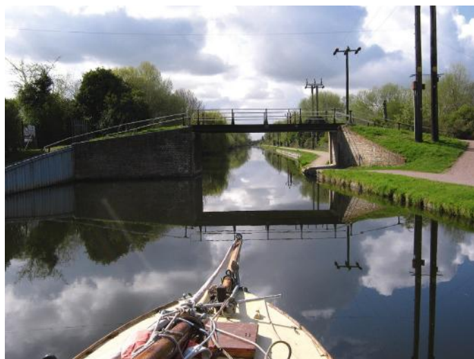
Mast, in tabernacle, lowers easily for passing under bridges when penetrating deep inland through canals and rivers
