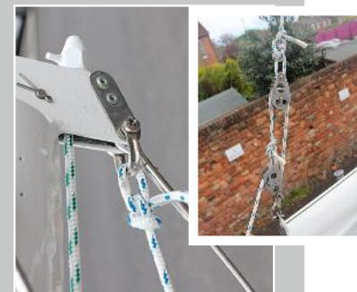
We attached a topping lift to a shackle on the backstay pin, with a tackle at the boom end (inset)
