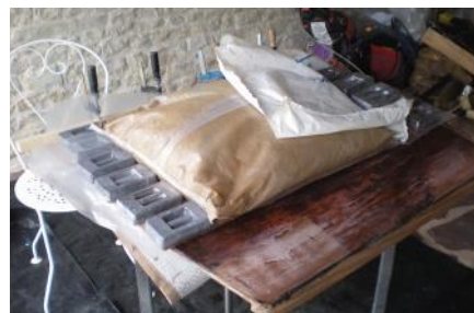
A bag of sand and divers' weights hold veneer down while the epoxy cures
