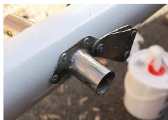
The spreader roots incorporate lower shroud attachments
