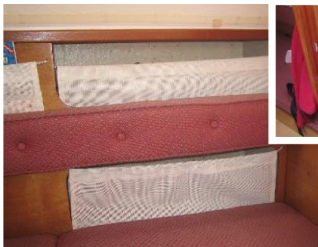
CAVE LOCKER FRONTS To stop everything falling out yet have complete access, simple PVC mesh panels have shock cord through the top hem and a piece of old wooden venetian blind spar along the bottom
