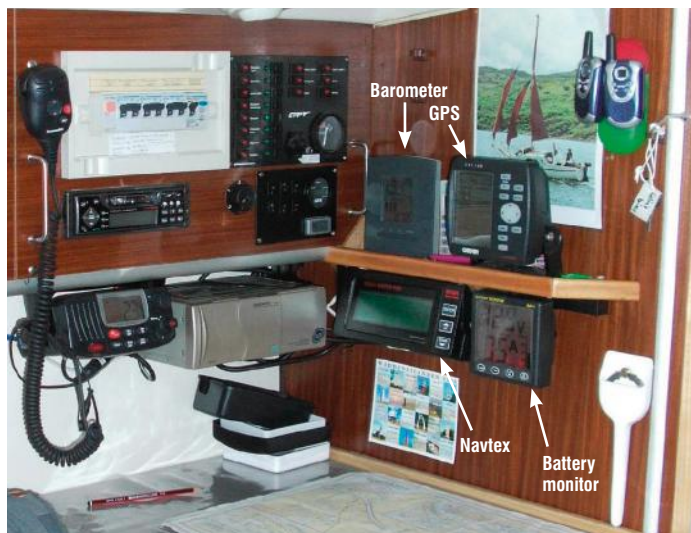
Colin's nav station with three primary sources of information clustered together: 'Where am I?' GPS; 'What's the weather doing?' Navtex and barometer; 'How much power is left?' battery monitor positioned where it can easily have an eye kept on it
