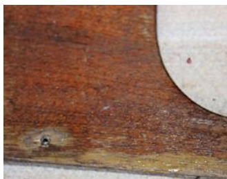
With varnish this damaged the only cure is to sand back to bare wood
