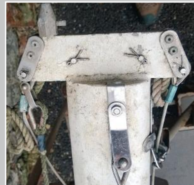
BEFORE: The spinnaker and jib halyards were led through a double block inside the forestay
