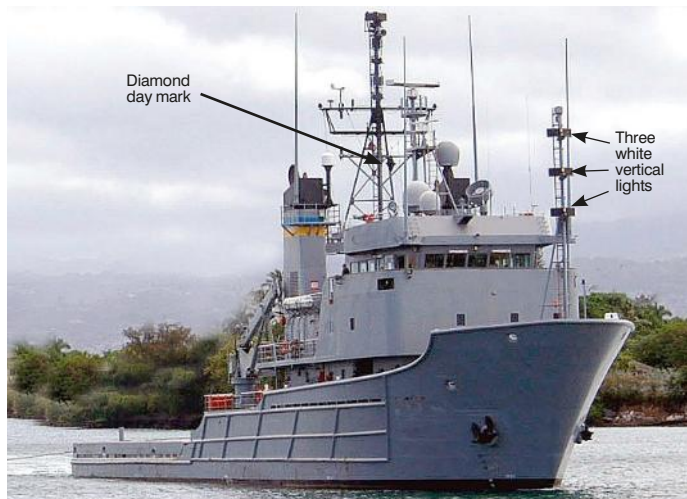
A diamond day mark can be hard to spot among the clutter on a tug's mast, but the three white vertical lights should be clearer
