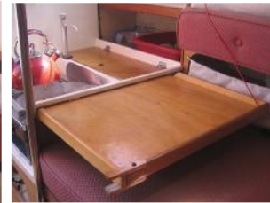
GALLEY TABLE Simply folds down to produce adequate work space for cooking. Also protects the settees from wayward galley produce when folded up
