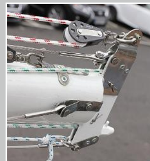
AFTER: The new setup, with a crane to project the spinnaker halyard forward of the forestay
