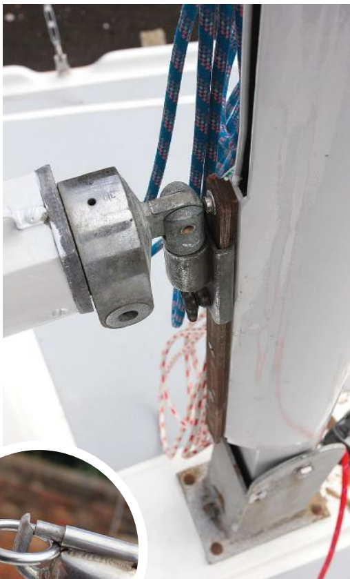
ABOVE The gooseneck sits on a Tufnol sliding track LEFT There is a sliding spinnaker pole track on the front of the mast
