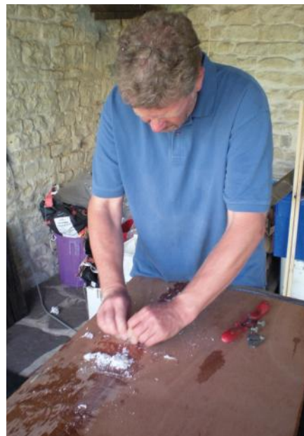
Scraping off the excess glue from the joins
