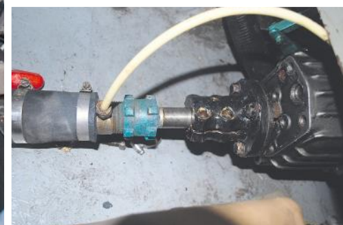
The existing stuffing box stern gland (with greaser tube) had worn grooves in the propshaft
