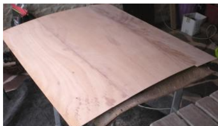
The glued veneer in place before trimming
