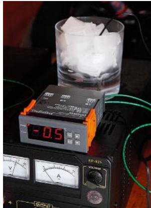
We used cubes of ice to confirm the accuracy of our temperature gauges
