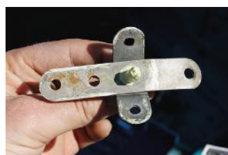
The tang for the jib halyard block comprises two stainless fittings
