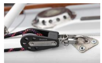
The spinnaker pole uphaul fitting is riveted onto the mast
