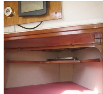
SALOON/COCKPIT TABLE Uses the same brackets and support for the table in the cockpit as in the saloon. Table stows beneath the foredeck
