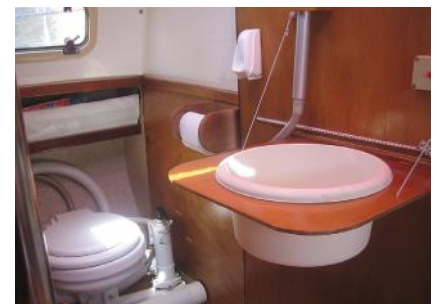
FOLDING WASH STAND With no room for a fixed basin, a washing-up bowl let into a plywood panel more than suffices. Water is from the tank via a manual lift pump and pours away down the heads
