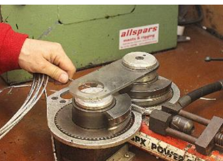
A hydraulic swaging machine attaches the shroud ends
