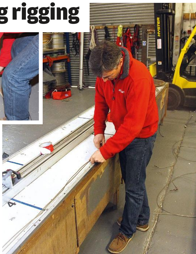
Andy measures our old shrouds in pairs before cutting them to length (inset)
