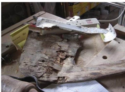
The old rudder blade and stock was beyond repair, so a new one was made: this is the new stock
