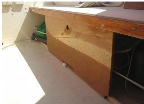
SLIDING COCKPIT LOCKER FRONTS Easy to slide or remove altogether, and everything is easily accessible. No leakage through cockpit seats either
