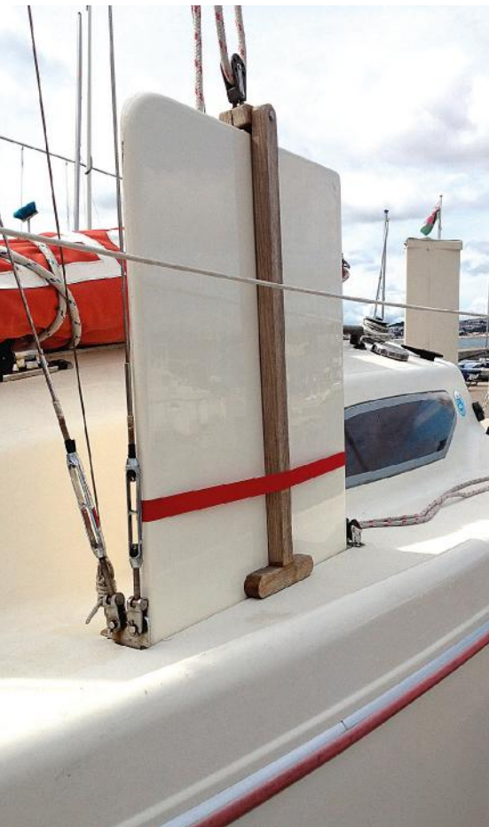
Peter proudly showed off his 'board-jacks' to hold the boards in place once the supporting rigging has been removed
