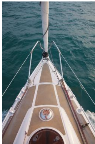
The tubular aluminium toerail and contrasting non-slip pattern were among Etap's trademark features on deck. There's even a ventilator
