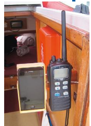
COMMUNICATION CENTRE iPhone holder made from a wooden blind glued to a 'Poppit' ball and socket mount so it can swivel or tilt. The folding arm is held in place with shock cord. Everything from music to Navionics charts right in front of you!
