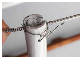
The shrouds are seized into grooves in the spreader ends
