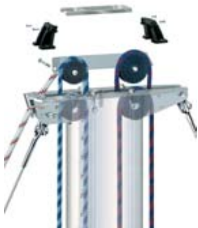
Remove any instrument base and the sheave separator. Lift out the sheaves for inspection. Replace the sheaves if necessary, and refit the separator.
