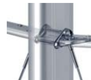
Through-bar spreader bracket, incorporates attachments for lower shrouds or intermediate shrouds.
